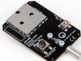
Triple LED lamp for student experiments to investigate additive and subtractive colour mixing.
