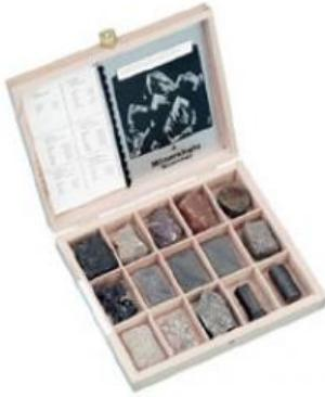
A collection of 15 samples in a wooden case 230 x 280 mm, with plastic inserts measuring 45 x 60 mm. The collection contains 15 selected, typical samples of raw materials, intermediate stages and final products in steel production. The collection is particularly suitable for explaining the blast furnace process and steel refining, since the progress from the raw ore to the ultimate steel products is shown quite clearly. The chemical composition is indicated for all specimens.
