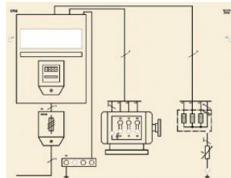
VP 8 Mask: TT-System, Dangerous voltage due to non permissible grounding with 2 ground electrodes
