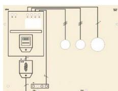
VP 4 Mask: TT-System with over current protection device To establish high voltage systems with a nominal voltage of up to 1000 V
