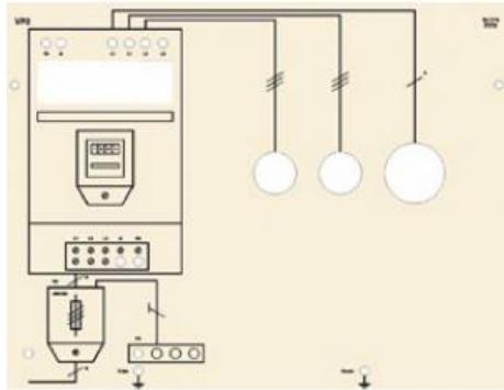
VP 2 Mask: TN-System with current failure protection device To establish high voltage systems with a nominal voltage of up to 1000 V
