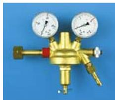
According to DIN, 2 pressure gauges, standard thread, fits gas bottle 661 013 as well as common commercial gas bottles, control range 0 ... 10 bar.
